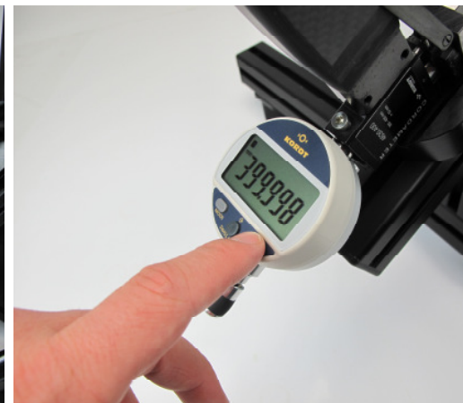
Set dial to „0“ or adjustment dimension
